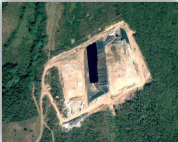
Fig. 3. Abandoned Landfill of Municipality of Veracruz, Veracruz State, Mexico in the year 2002, with cell 1 and cell 2 closed and cell 3 in use.
