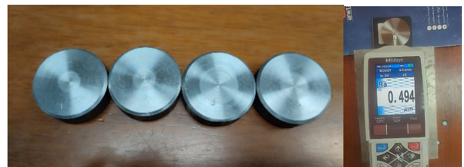
Fig. 1. Machined specimens and experimental measurement of surface roughness
