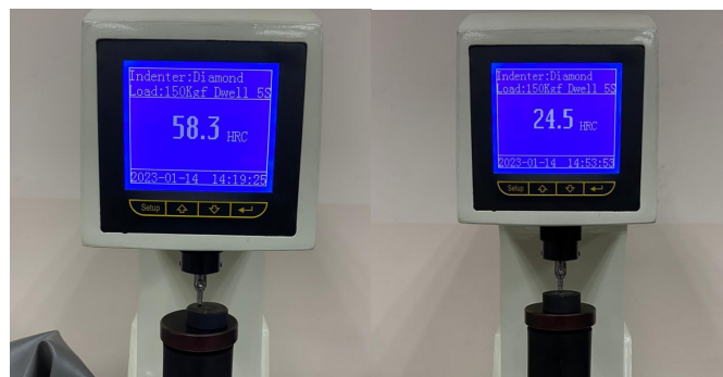
Fig. 4. Surface hardness measurements with carburizing in coking coal and charcoal
