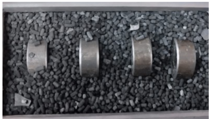
Fig. 2. Hermetic box for carburizing
