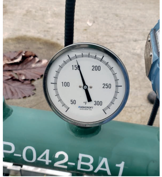
Fig. 8. Ashcroft Bimetallic Thermometer.
