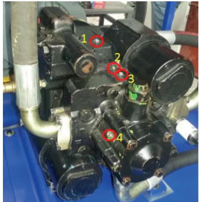
Fig. 3. Positions taken for vibration measurement.
