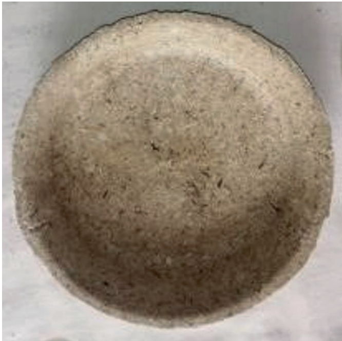
Fig. 10. Prototype of a plate made from sugarcane bagasse.
