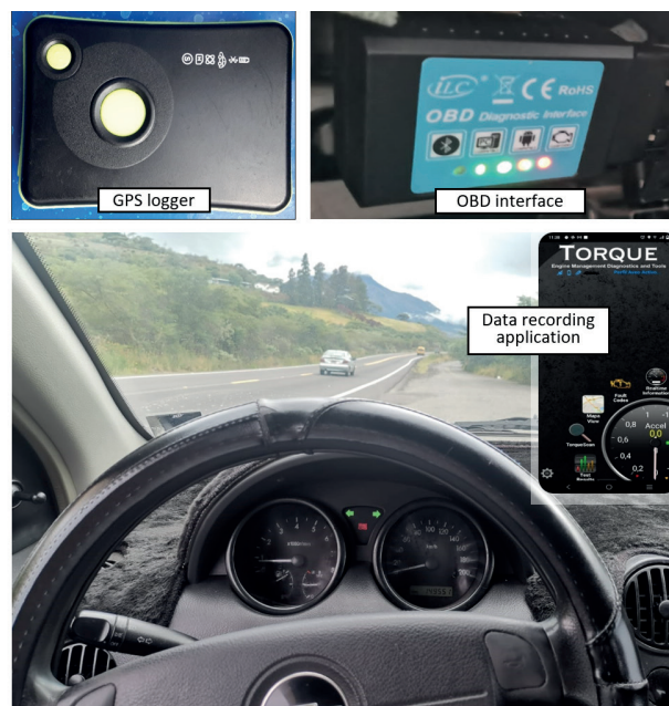
Fig. 2. Tested vehicle equipped on board with GPS logger, OBD interface, and OBD data recording application for field data collection.
