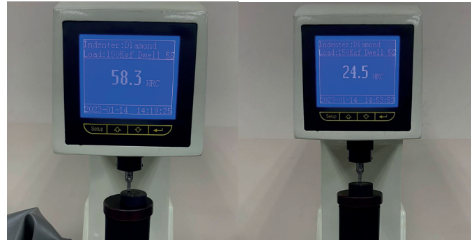
Fig. 4. Surface hardness measurements with carburizing in coking coal and charcoal
