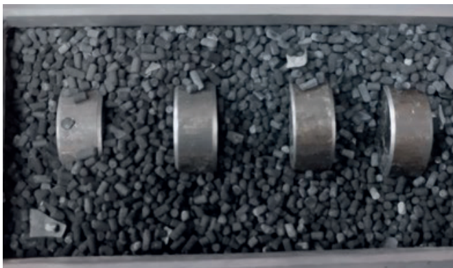
Fig. 2. Hermetic box for carburizing
