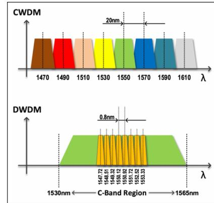
Fig. 6. CWDM Channels vs. DWDM channels [15].
