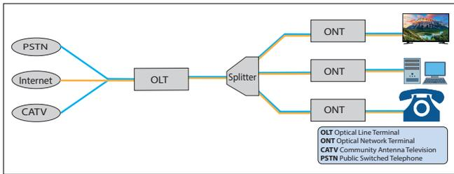
Fig. 1. Structure of a PON network, based on [5].
