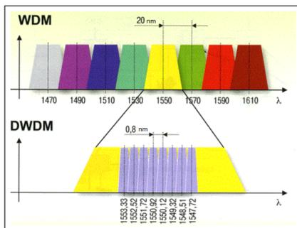
Fig. 5. WDM Channels vs. DWDM [19].
