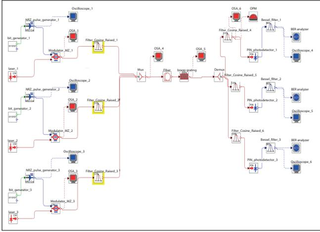
Fig. 14. Simulation using a Raised Cosine Filter.
