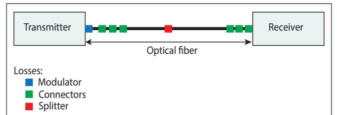
**Fig. 10.** Loss diagram of the optical link.
