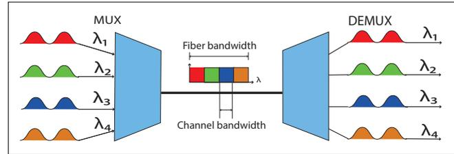
Fig. 2. Multiplexing and demultiplexing in WDM, based on [12].
