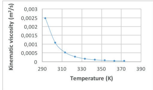
Fig. 5. Kinematic viscosity of heavy crude oil.
