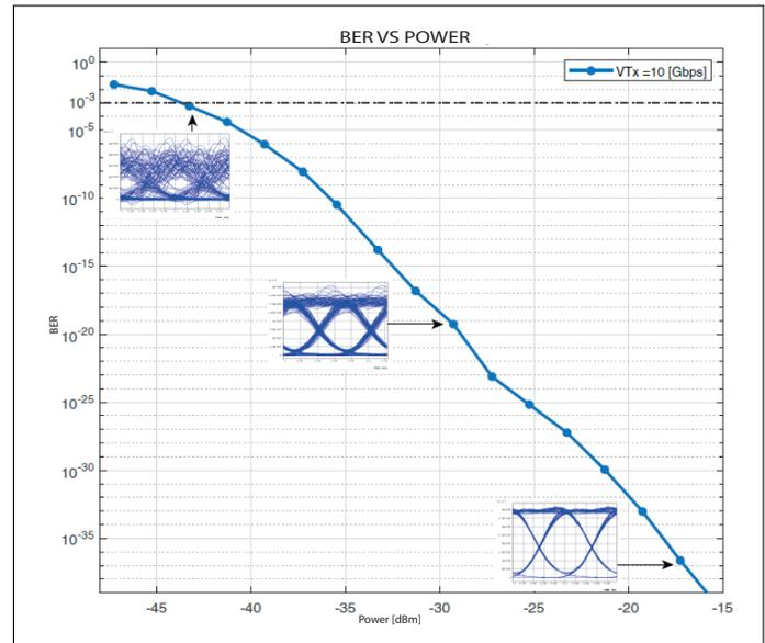
Fig. 25. BER vs. RECEIVED POWER and 25GHz channel spacing.
