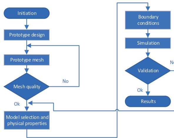
Fig. 1. Methodology used in the CFD simulation [12].
