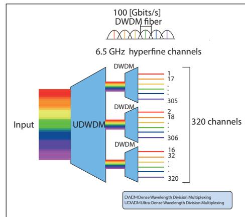
Fig. 7. 320 channels UDWDM transmission, based on [18].
