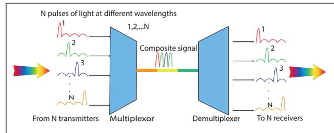
Fig. 3. Multiplexing and demultiplexing in CWDM, based on [14].
