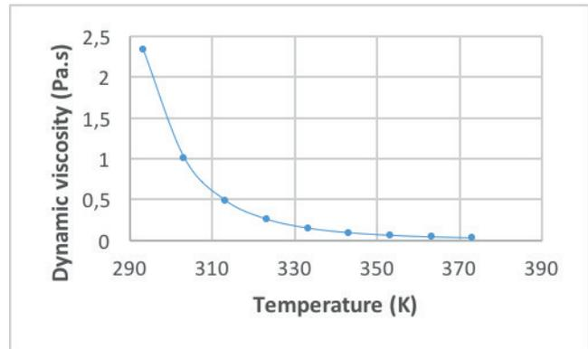
Fig. 6. Dynamic viscosity of heavy crude oil.
