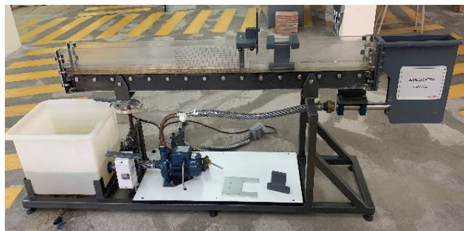
Fig. 1. Sediment Transport Demonstration Channel (Sedimentation Channel Operation Instructions, 2004, Cussons brand).
