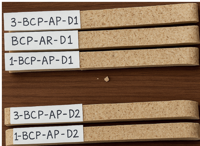
Fig. 3. Specimens for the flexural test.
