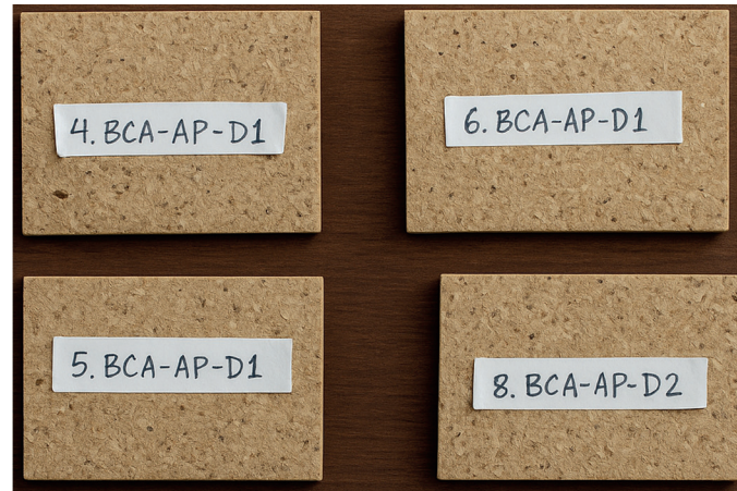
Fig. 4. Specimens for the impact test.
